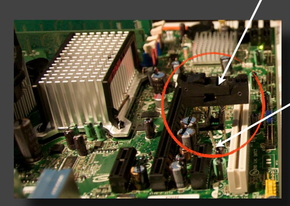
Extra socket soldered to the motherboard (special thanks to **Piotr Witczak**, AVT
